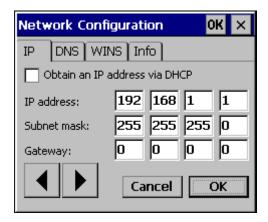
It is always possible for the device to obtain an IP address (network address) via a DHCP server on startup **«Obtain an IP address via DHCP»**. However, for the device to have a unique ID, you should select **«Specify an IP address»**.
